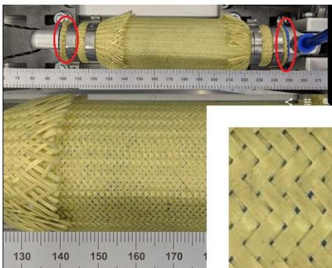
Fig. 1 Assembly of an untethered hydraulic actuated muscle.
