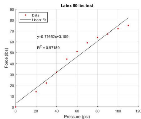
Fig. 2 Relation between force and pressure.
