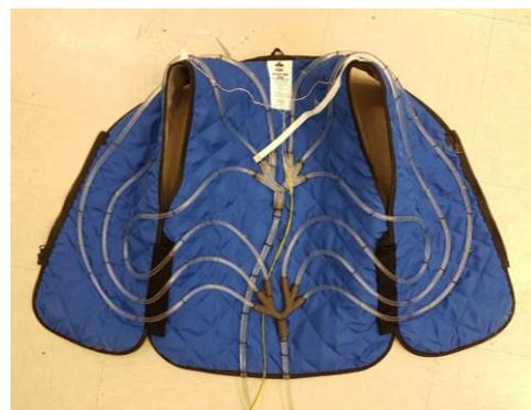
Figure 4, Tubes and water junctions sewn onto inside surface of the vest.
