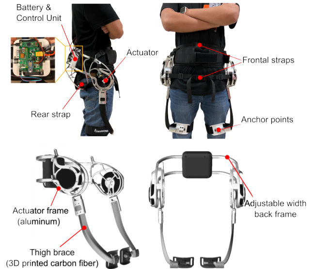
Fig. 1. Our new proposed portable hip exoskeleton consists of two quasi-direct-drive actuators, adjustable width back frame, multi-strap wearable, and compact electronics. This design reduced wobbling (relative angular velocity between the human and robot) by 74% compared to a traditional configuration.
