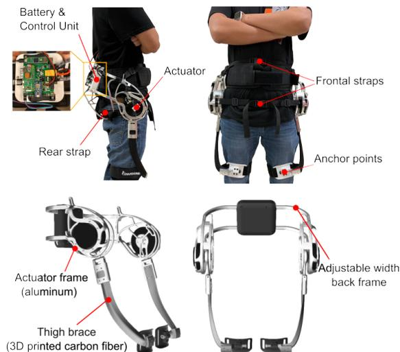
Fig. 1. Breakdown of the mechatronics design of our hip exoskeleton. Singular control box is needed as the electronics and battery is contained within making the mass more central and less noticeable.
