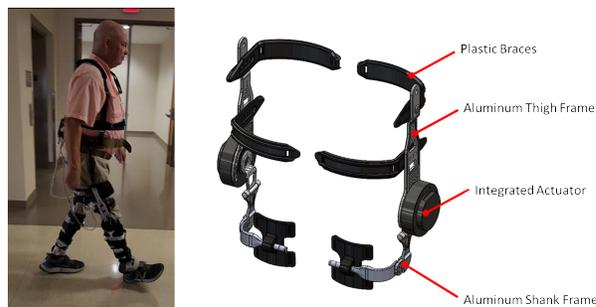
Fig. 2. Mechanical design of our portable knee exoskeleton. The knee exoskeleton was able to provide walking assistance to an elderly subject
