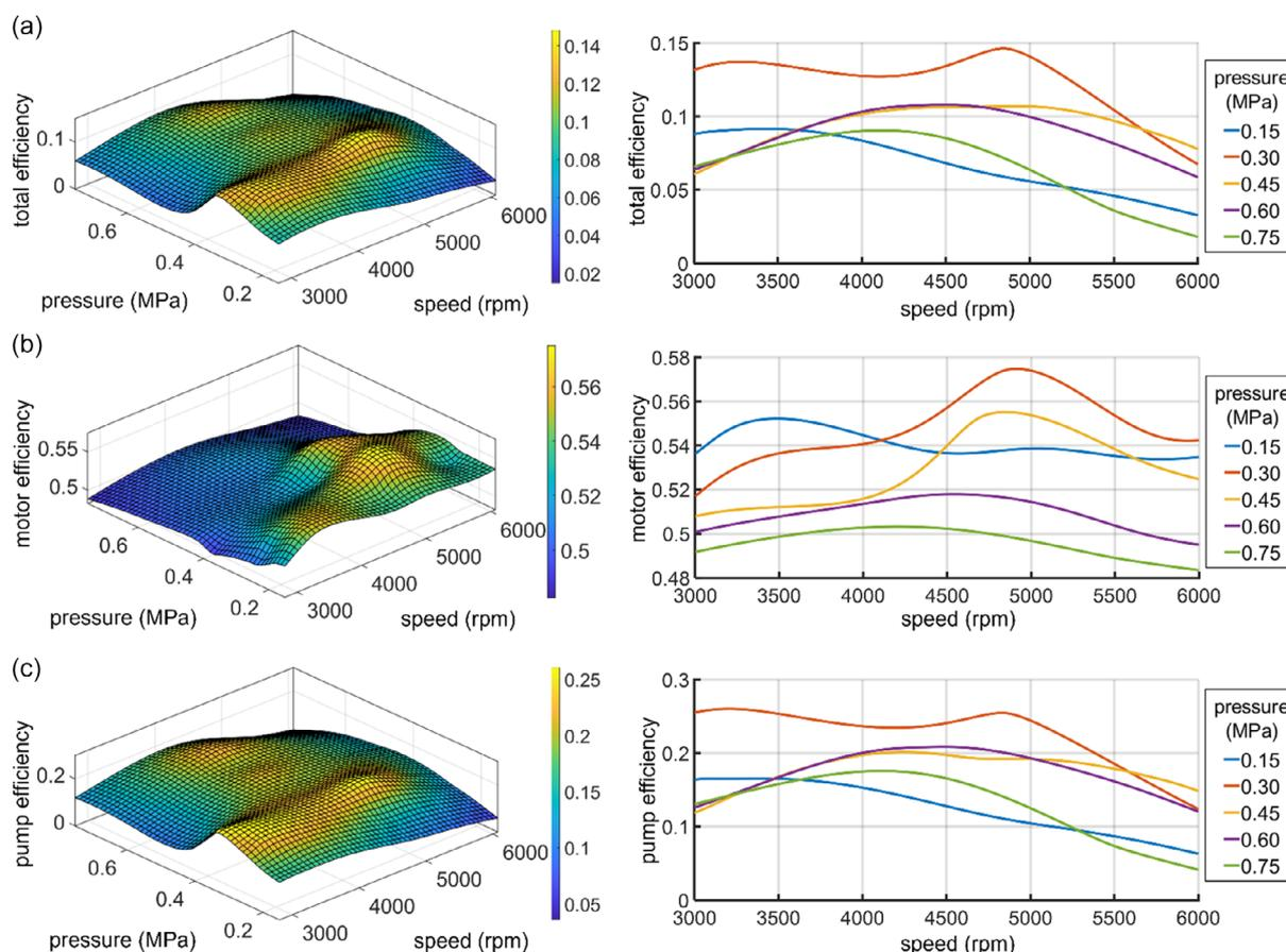
**Figure 6.** a) Our developed mechatronic system achieved relatively high efficiency thanks to the high contributions of b) motor only and c) pump only. A maximum value of about 15% is recorded at 0.32 MPa and 5000 rpm, which is comparably higher than peak efficiencies reached by other state-of-the-art systems on a similar scale.
