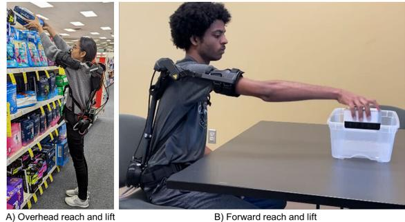
Fig. 1. (A) Our portable exoskeleton can be used outside a clinical setting. The exoskeleton is able to provide assistance to reach and lift a mass over the head. (B) The exoskeleton is able to provide assistance in a variety of manual tasks, such as a forward reach and grab.
