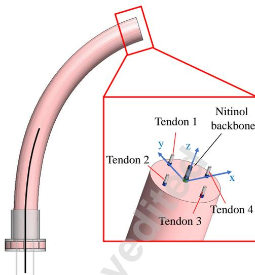
Fig. 1. Design of TDCT soft robot with a super-elastic retractable Nitinol tube (black curve) for stiffness modulation. 4 tendons are symmetrically located at the cross section with the same distance to the center. The Nitinol insertion can be achieved manually (in this paper) or via precise linear motors. Noting that friction-reducing sleeves are integrated with the soft robot to reduce the friction between the soft robot and tendons/Nitinol tube.
