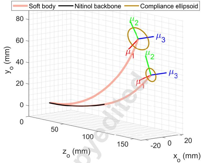
Fig. 10. CE projected in  $\boldsymbol{\mu}_2 - \boldsymbol{\mu}_3$  plane with various Nitinol backbone insertion and constant tendon tension, where  $\boldsymbol{\mu}_1, \boldsymbol{\mu}_2, \boldsymbol{\mu}_3$  are eigenvectors of CM. The dimension of the CE becomes smaller with Nitinol backbone inserted, indicating the stiffness of the TDCT soft robot tip is enhanced.
